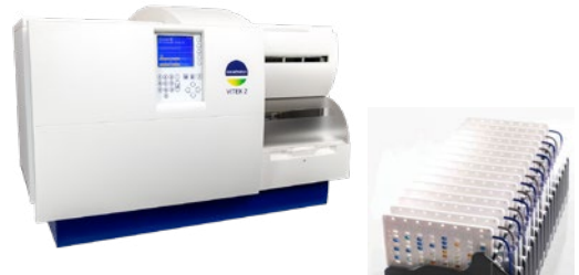
Figure 16. VITEK® 2 instrument and ID/AST cards
